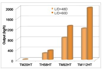
to our experience with the TPV's, we have ascertained that a machine longer than 48D (which is the usual standard for the production of TPE) preserves the quality (or even, in some cases, improves it) and increases the output. A longer machine improves the entire management of the process parameters as the screw profile, the thermal profile and the screw r.p.m., achieving the optimal dispersion and crosslinking.
