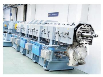
The test done at our Technological Center with the Lab. twin-screw "reactor" extruder was giving promising results. This was also possible due to our previous experiences in "reaction extruders" for other kind of process, always starting from liquid monomers for obtaining the proper reaction and a good polymer.
