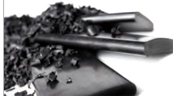
The thermo-mechanical devulcanization is possible as S-S, C-S and C-C bonds have different energy, which is respectively of 370, 310 and 270 kJ / mol. Thanks to the appropriate combination of thermal and mechanical energy, it is possible to selectively break S-S and C-S bonds.
